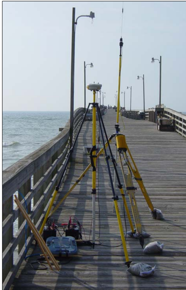
Figure 8. RTK GPS base station set up on the Jolly Roger fishing pier.
