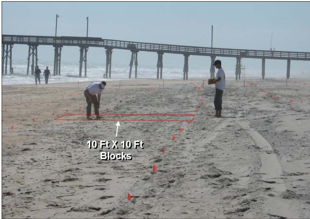
Figure 13. Layout of survey area to quantify the amount of clasts > 3” in diameter within a 50,000 ft 2 area of Topsail Beach. Wooden stakes around the perimeter of the survey area and utility flags mark the corners of 10 ft x 10 ft blocks.
