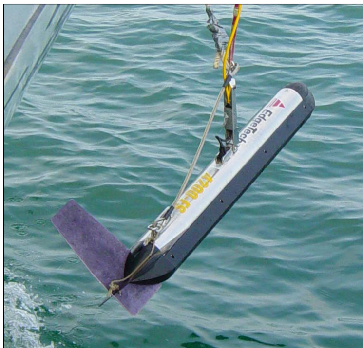
Figure 9. Deployment of the EdgeTech 4200-FS sidescan sonar towfish.
